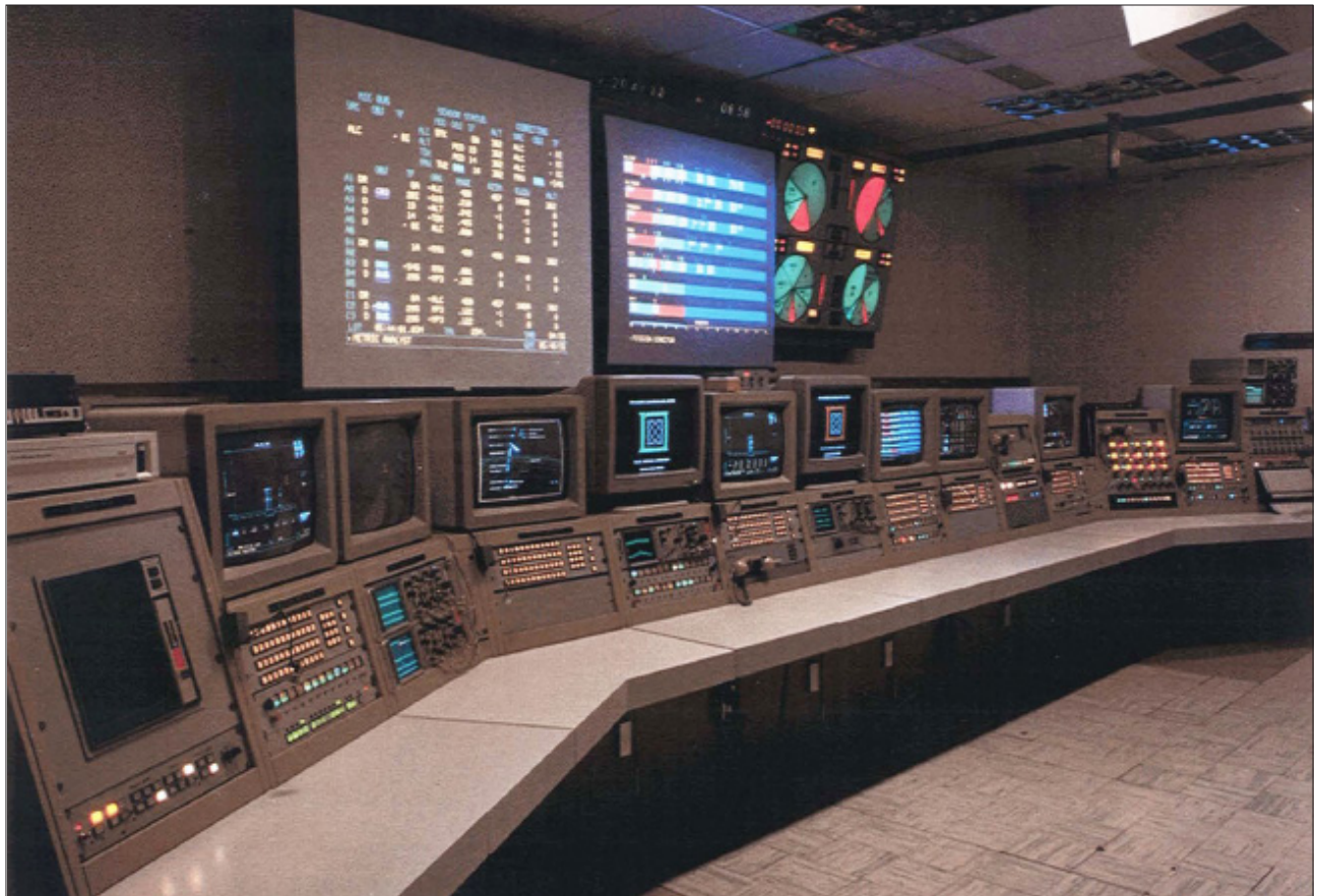
FIGURE 9. The KREMS Control Center, depicted here, managed all three radars, while providing cross-platform correlative and corroborative data.
