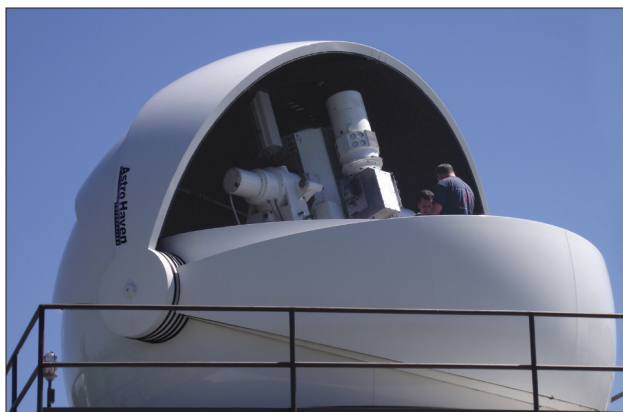
FIGURE 17. The Super RADOT optical sites at Kwajalein are being upgraded with new domes and camera systems.
