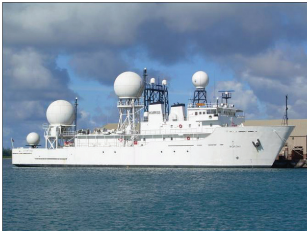
FIGURE 15. The Kwajalein Mobile Range Safety System monitors theater-class missile launches from its ship-based platforms.
