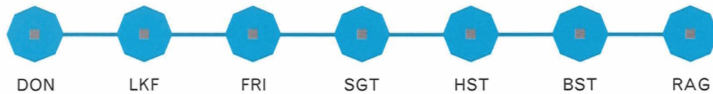
FIGURE 9. Simulation of the TRAMCON system for the Digital European Backbone II-A (DEB II-A). Used by the Department of Defense as its mainstay transmission system in Europe, DEB II-A is a microwave radio network with strings of mountaintop repeater stations providing backbone interswitch trunk circuits for voice and data networks. The simulation shown here is for a segment of DEB II-A in Germany, beginning at Donnersberg (DON), continuing through Langerkopf (LKF) and Stuttgart (SGT), and ending at Reese-Augsburg (RAG).
